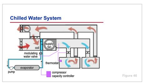
In contrast to the DX system examples shown previously, a chilled-water system responds to changing space loads by controlling the capacity of the chilled-water cooling coil. Although there are various methods of controlling the capacity of this coil, this discussion will assume the use of a modulating water valve.
